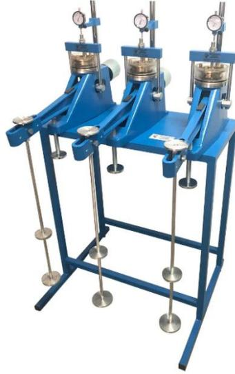
Front Loading Oedometer (consolidation), cast aluminium frame, the lever arm incorporates 9:1, 10:1 and 11:1 beam ratios.
